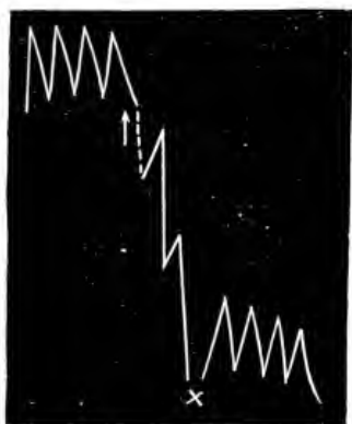
FIG. 73. Effect of HCl Vapour Arrow indicates moment of application. Depressing effect neutralised by antagonistic action of \text{NH}_3 at x.
