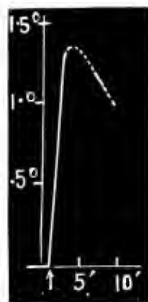
FIG. 269. Torsional Response of Complex Strip of Ebonite and India-rubber under Lateral Action of Strong Radiation
