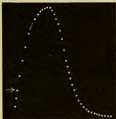
FIG. 220. Effect of Formaldehyde applied at arrow, showing preliminary acceleration followed by reversal. A preliminary portion of the record is omitted. Successive dots at intervals of 3 minutes.
