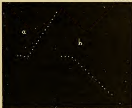
FIG. 10. Record showing (a) condition of overbalance, and (b) underbalance of growth. (Magnification 2000 times.)
