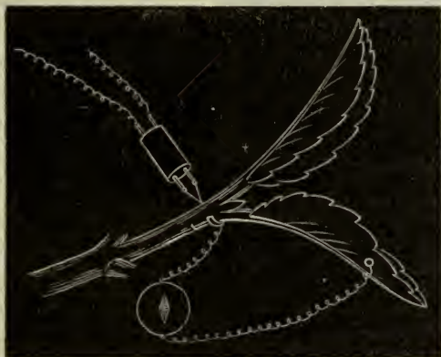
FIG. 233. Experimental Arrangement for Detection of Electrical Change induced at the Point transversely Distal to Point stimulated
