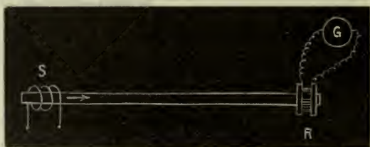
FIG. 371. Experimental Arrangement for obtaining Response in Iron by Induction Current
