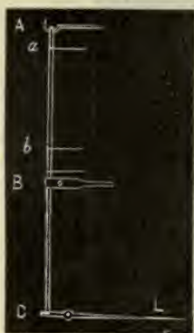
FIG. 315. Diagrammatic Representation of Arrangement for Obtaining Transmitted Effect of Stimulus. L, indicating lever
